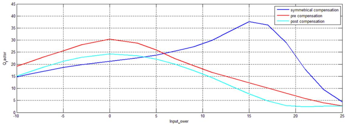
**Figure 8:** Comparison of Transmission influence of three compensation scheme
