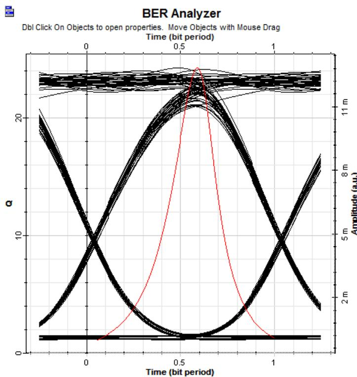
Figure 7: Eye diagram of post compensation scheme.
