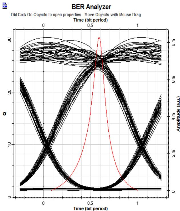
Figure 6: Eye Diagram Of pre Compensation Scheme
