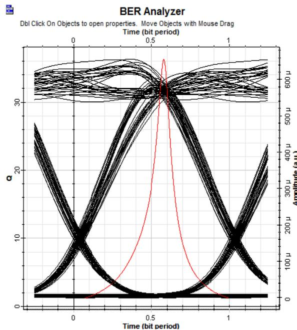
**Figure 5:** Eye Diagram of Symmetrical Compensation Scheme
